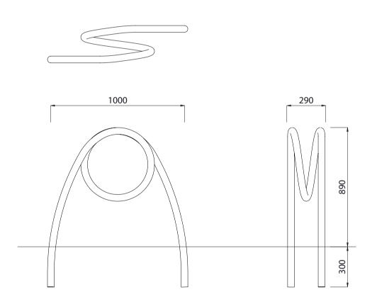
MATERIALSFINISHESFINISH OPTIONSSteelwork• 316 Stainless steel as standard• Electropolished or<br/>Buff polished (hand rubbed satin finish) or<br/>Bead blasted• Custom paint optionsOPTIONSDIMENSIONSWEIGHT• Plant mounted as standard• 1000L x 890H x 290W• 8Kg
