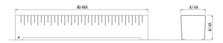
**FINISHES FINISH OPTIONS MATERIALS** · Custom Paint options Powdercoated Metalwork Aluminium as standard Hardware / Fasteners Stainless steel **OPTIONS DIMENSIONS** WEIGHT • 600L x 450H x 450D • 12KG Custom laser design • 1800L x 450H x 450D • End panels • 35KG
